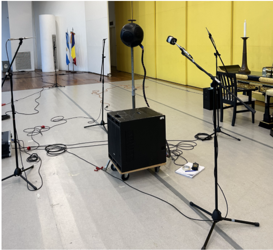
Figure 13: Measurement of stage parameters.
